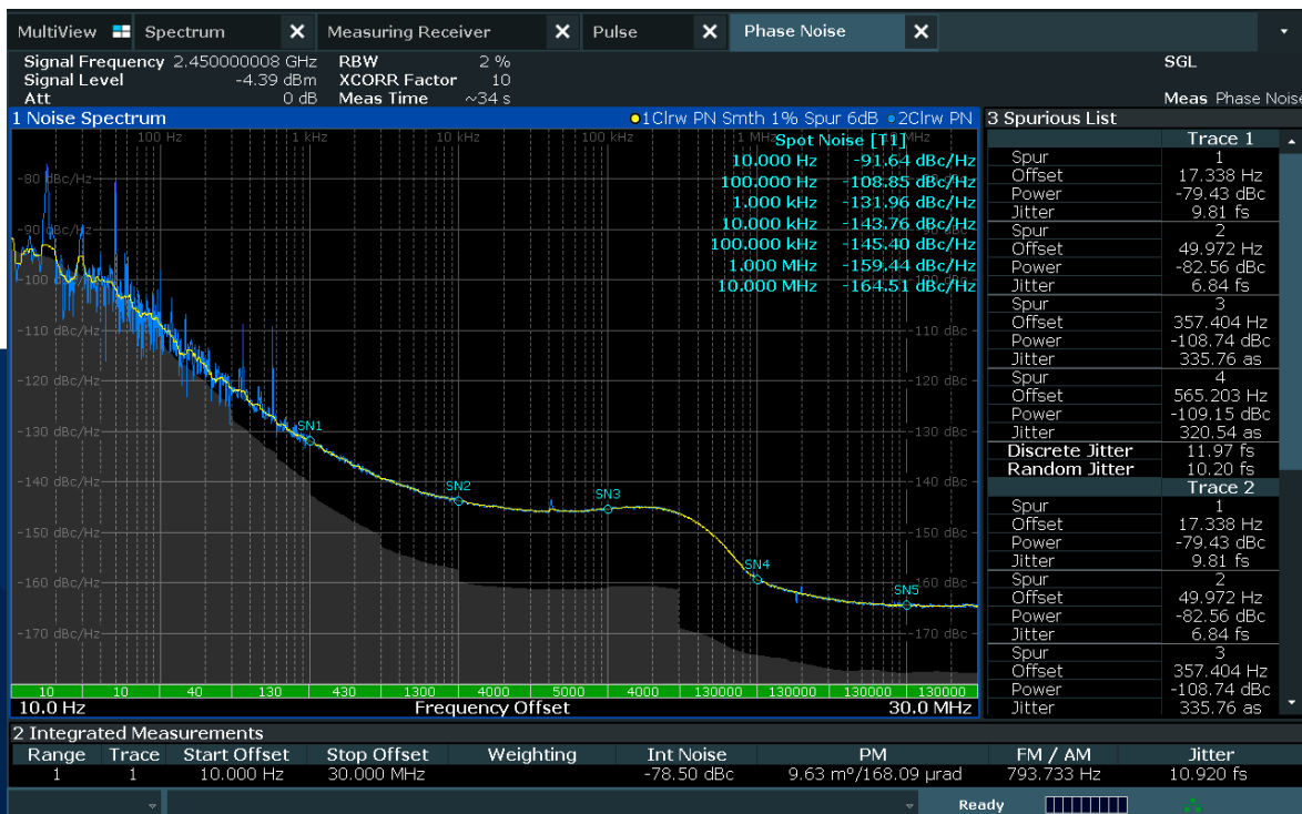
Measurement of amplitude and phase noise with the R&S®FSMR3-B60 option.
